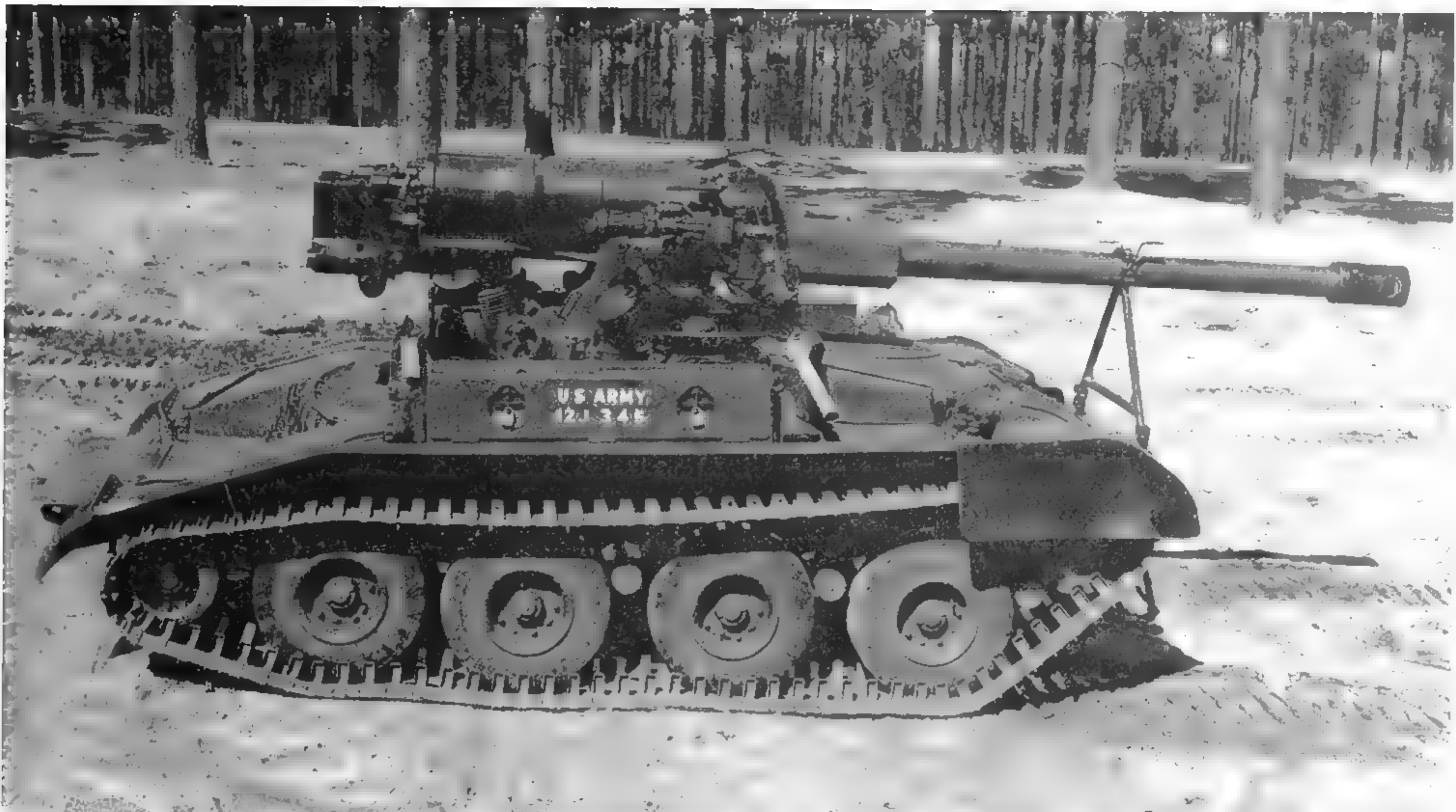
The M56 exhaust stack was routed out almost directly under the gun shield, and the deck at the rear of the hull served as a platform for the loader. In this view the gun tube is properly secured for travel.
